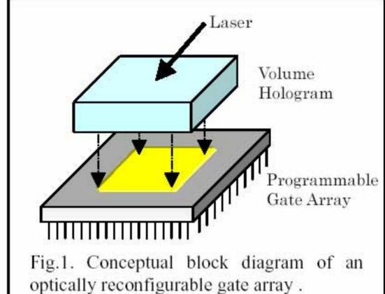
In this scheme, an optically reconfigurable gate array (ORGA) is developed to overcome the slow configuration time. The conceptual block diagram of the ORGA is illustrated in Fig.1. The configuration data stored in a volume hologram is written optically in a 2D onto each of the on-chip photodetectors of the programmable gate array. As the result, the ORGA can achieve very fast parallel configuration and reconfiguration.
