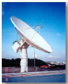
CRISP's 6-m X band antenna for MODIS data reception
